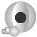
The microspheres in the HY-TECH insulating ceramic additive have compressive strengths up to 60,000 psi, a softening point of about 1800° C., and they are fairly chemical resistant, with low thermal conductivity of 0.1 W / m / Deg. C.
