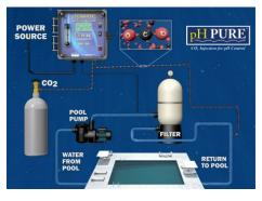
A new product that keeps the pool balanced around the clock virtually without the need of chemicals - including muriatic acid. Economically and safely used on commercial pools for decades, the system injects CO<sub>2</sub> – carbon dioxide into the pool. It's about 1/5th the cost of using muriatic acid and sodium bicarbonate.
