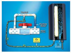
An ultra-violet ozone system compete with a Venturi manifold setup that alone will reduce chlorine use up to 50% or up to 95% when used in conjunction with the **MineralPURE** ionizer. Enjoy crystal clear water. A great oxidizer and effective in controlling cryptosporidium and E. coli.
